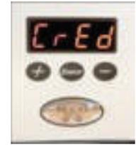
\*1.9- To read the steps, we have to be with the mill at rest and press both the (+) and (-) and (step) buttons at the same time and then the number of these
