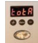
**1.6-** (Cred) here we can manually modify (without introducing coins) the credits that the machine has, we can either give you services or remove it, only using the (+) or (-) buttons
